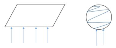
If there was no air resistance (friction), then both the sheet of paper and crumpled ball of paper would have fallen at the same time.
