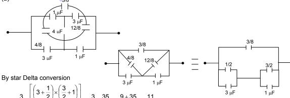
$$C_{\text{eff}} = \frac{3}{8} + \left[ \frac{\left(3 + \frac{1}{2}\right) \times \left(\frac{3}{2} + 1\right)}{\left(3 + \frac{1}{2}\right) + \left(\frac{3}{2} + 1\right)} \right] = \frac{3}{8} + \frac{35}{24} = \frac{9 + 35}{24} = \frac{11}{6} \ \mu\text{F}$$
