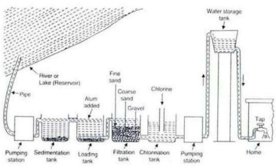
Fig. Water purification process at water works
