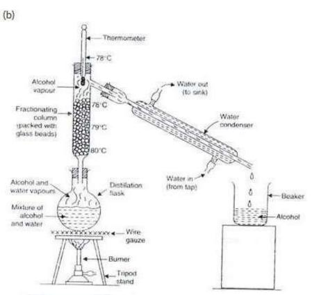
Fig. Separation of mixture of alcohol and water by fractional distillation
