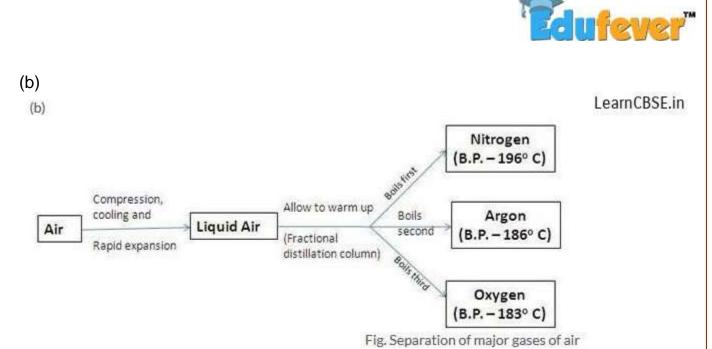
Fig. Separation of major gases of air
